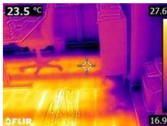
Figure 60: Heat radiating through floorboards from distribution pipework below – Image © Landsverk
