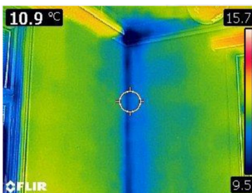
Figure 38: Heat loss at and above the wall junction at a corner of the ground floor – Image © OAMK
