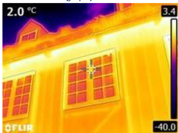
Figure 57: Heat loss at eaves below fascia boards and via timber joints – Image © Landsverk
