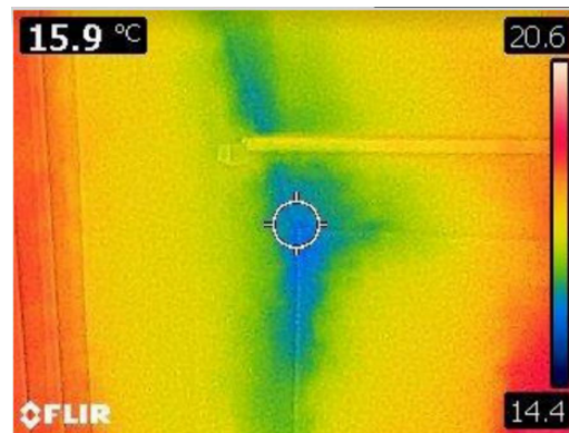
Figure 41: Heat loss via a stud wall junction in a 1 st floor cupboard – Image © OAMK
