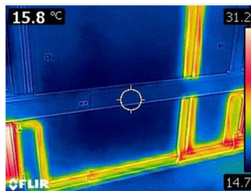
Figure 42: Heat loss in the middle of an external wall on the ground floor – Image © OAMK
