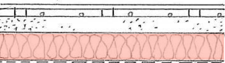
Excavated & new ground floor slab with underfloor heating & floor finish
